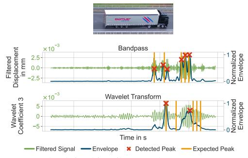
Figure 9. Example result of a truck for our filtering approaches.
