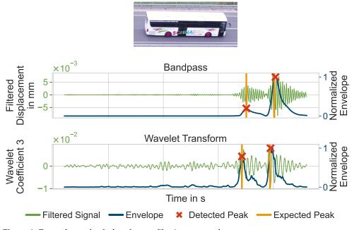
Figure 8. Example result of a bus for our filtering approaches.
