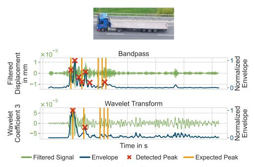
Figure 10. Second example result of a truck for our filtering approaches.
