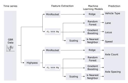
**Figure 5.** Methodology for our feature-based methods. *F*1–*FN* represent manually extracted features. We use a high-pass filter before feature extraction for the axle counting and axle spacing estimation.
