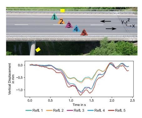
**Figure 2.** Overview of the bridge and an example displacement time series. The yellow rectangles in the upper image represent the GBRs, and the numbered triangles represent the five reflectors at their approximate position.
